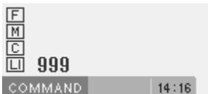
5. Move the work clamp with  $\Delta \nabla \triangleleft \triangleright$ . Press **L** when the needle point is at point D of the pattern.
