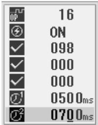
4. Write the option program over the program on the CF card of the sewing machine. Press
