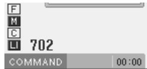
4. Input the zigzag stitch length in 3 digits, and then press **M**.
