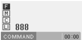
4. Input the magnification in 3 digits in the X direction, and then press **F**.
