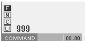
4. Input the magnification in 3 digits in the X direction, and then press **F**.
