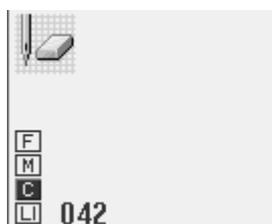
Input    to delete data after the current needle position.
