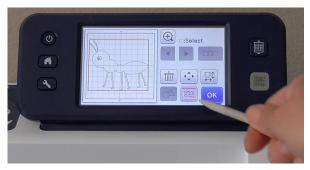
**step 4.** Apply the Iron-On Transfer Film onto the mat with the film side up. Insert it into the machine and click on the "Scan" button.
