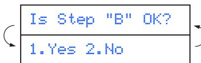
Check the 600 dpi and 1200 dpi test print to see if **No.5** most closely matches the OK sample (**No.0**). Press **1** if **No.5** matches it.
